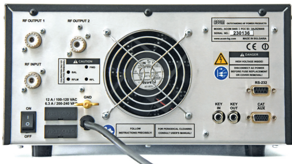
Figure 4 — The rear panel, showing the cooling fan and available connections.
