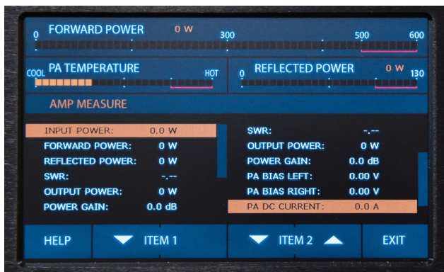
Figure 3 — The AMP MEASURE screen is used to select the parameters displayed in the bar just above the band display.
